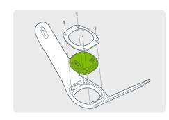
The icon is removable with the help of a small screwdriver under adult supervision. Be sure not to over-tighten the screws.
